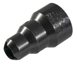
From Klein Tools, the Conduit Reamer works with a screwdriver to ream and smooth thin-wall conduit. It locks onto a screwdriver and can ream both ID and OD at the same time. Comes with two set-screws to fit either round or square-shank screwdrivers.
