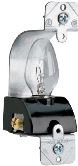
Designed to give adequate light when installed behind a louvre plate or indicator jewel. Mounts in standard wall box. Plate mounting is 2 3/8" and 3 13/16". UL listed for 120 VAC circuits. Plate not included. Standard lampholder 4 watt.
