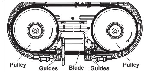
5. To install a blade, press the blade between the guides, then fit it around the pulleys.
