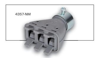
**The 4357-NM** transitions multiple nonmetallic cables into 3/4" EMT. Simply squeeze the tabs to install or remove the cables. They're perfect for prefabrication of bundles of nonmetallic cable.
