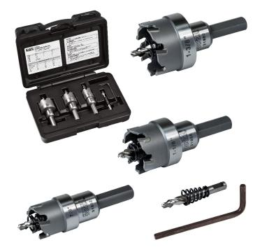
This 4-piece Carbide-Tipped Hole Cutter kit cuts quick, precise holes in a variety of materials. Set includes three commonly used sizes plus an extra pilot bit. Integrated flange prevents the operator from drilling beyond the sheet metal. Split point pilot drill bit prevents bit walking.
