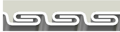
Interlocked Design 1-1/2" through 4" with no bonding wire
