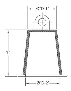
Poly Plugs with Pulling Eyes are designed for the temporary sealing of conduit to protect the duct from the effects of weather, job site debris, and animal damage. The molded in pull-eye is used to secure excess pulling rope within conduit.
