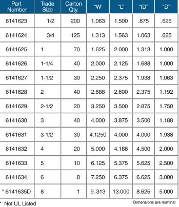
Schedule 40 Standard Center Stop Couplings are used to join lengths of conduit pipe together with two solvent weld socket ends.
