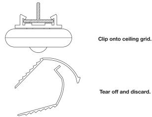
To install on a suspended ceiling panel:
