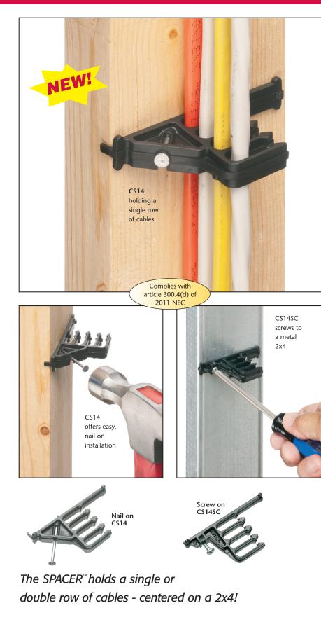
The SPACER<sup>™</sup>, Arlington's new, non-metallic Cable Spacer holds power or low voltage cable secure and centered on a 2x4. Perfect for routing, fastening and positioning power or datacom cable, it holds a single or double row of *up to eight* cables securely between the forks.
