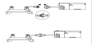
Place driver box into ceiling. (Optional: Mount using mounting tabs and screws)
