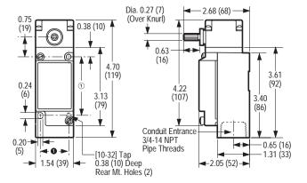
① Can accommodate both U.S., 1.16 (29.4) x 2.34 (59.5) and DIN, 1.18 (30) x 3.26 (60), mounting dimensions.
