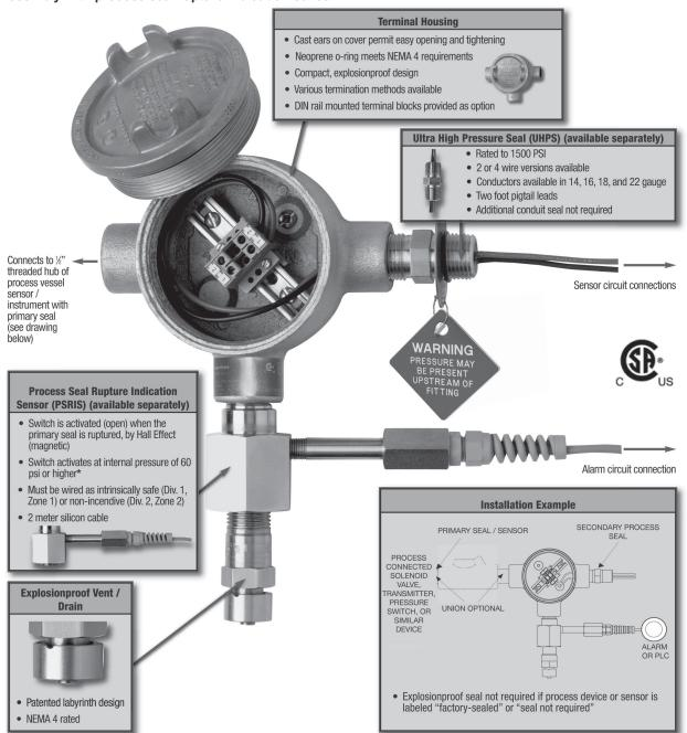
\*60 psi internal pressure rating at 25°C ambient. Activation pressure may vary +/ - 10% depending on ambient variation.
