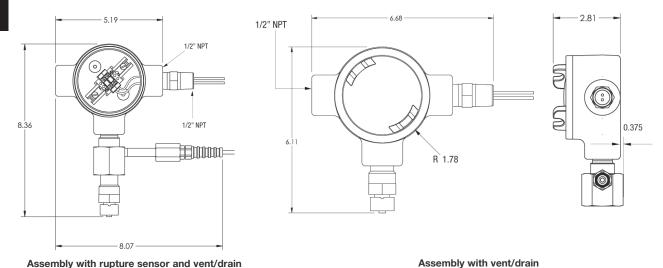
Assembly with rupture sensor and vent/drain
