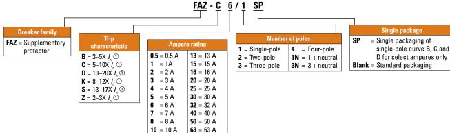
①  $I_p$  = Rated current for instantaneous trip characteristics.
