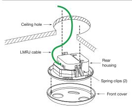
Mount directly to ceiling tile using spring clips (included) or to a 4" octagonal box. See installation instructions for more details.
