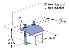
Design Load Each 1000 Lbs (4.4 kN) Use in Pairs Only
