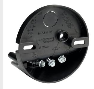
Ceiling Fan Box with Direct Mount. Suitable for Single or Double Joist. Easy installation. One #10 x 1 1/4 inch screw holds the box at rough in. Two factory-supplied #10 x 2 inch screws secure the fan or fixture through the box, directly to the joist. UL Listed for fan and fixture support.
