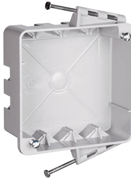
4" Square Box with threaded mounting holes, captive mounting nails each end. 3 Auto/Clamps each end, 2 on side opposite to nails. Two #8 Mounting Screws Factory Installed.
