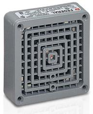
Model 350 Vibratone® Horn produces a loud tone by the electro-mechanical vibration of a diaphragm. Its compact size, loud output and heavy-duty construction makes Model 350 ideal for industrial and institutional signaling applications. It's popularly used for general alarming, start and dismissal noticing, coded paging and process control in noisy areas.
