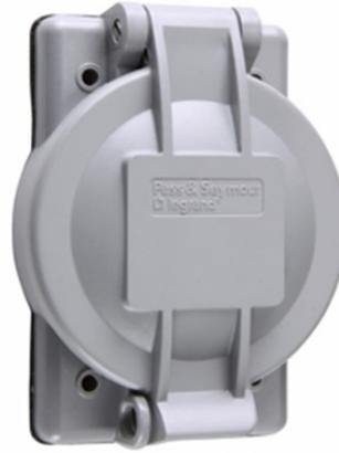
Industrial Grade Weatherproof Lift Cover For Flanged Inlet/Outlet, 1.96" Diameter Opening to Accommodate 15/20A Straight Blade, 15A Turnlok, 20403 Power Interrupter, Gray
