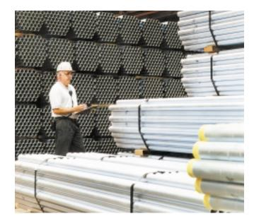
Galvite® Rigid Steel Conduit is manufactured in standard trade sizes through 6". Please refer to the chart on the reverse side of this data sheet for complete dimension and weight information. Inventories of our Rigid Steel Conduit are maintained by leading distributors throughout North America.
