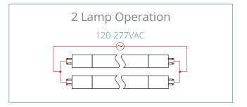
**NOTE**: both pins on each end of lamp must be connected to line voltage as shown above. If lamp holder is a "non-shunted" (T12) type, it must be shunted (shorted) by external jumper. Most T8 lamp holders are internally shunted and will not require an external jumper.
