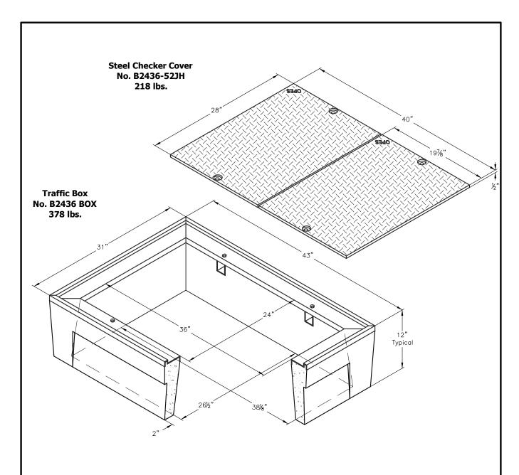
A high density reinforced concrete box with non—settling shoulders positioned to maintain grade and facilitate back filling. Hex—Head Bolts are included with Box. Approximate dimensions and weight shown.
