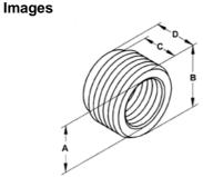
Download Photo Image Dow Dimension A in Inches: 5/8 Dimension B in Inches: 7/8 Dimension C in Inches: 7/16 Dimension D in Inches: 9/16
