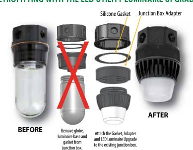
NOTE: Please see Installation Requirements for the ProSeries LED Utility Luminaire and LED Upgrade shown on page 89.
