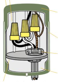
SpliceCap compartment fully encloses and protects the circuit conductors from moisture, dirt and abrasion.
