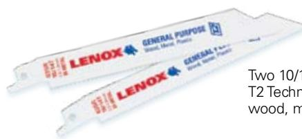
Two 10/14 TPI General Purpose reciprocating blades featuring T2 Technology. The 0.035" thick blades are ideal for cutting wood, metal and plastic 12129635R, 12130835R
