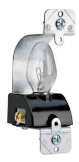
Designed to give adequate light when installed behind a louvre plate or indicator jewel. Mounts in standard wall box. Plate mounting is 2 3/8" and 3 13/16". UL listed for 120 VAC circuits. Plate not included. Standard lampholder 4 watt.
