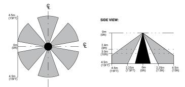
Note: Installation of integrated sensors within 3-ft (1m) of HVAC air vents is not recommended. The pattern shown is intended solely as a general guide and is not to scale.
