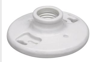
Medium base, porcelain, one piece keyless. 2 terminals with tri-drive screws, fits 3 1/4" and 4" boxes, with cage neck.
