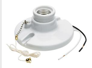
Medium base, porcelain, pullchain, 2 terminals with tri-drive screws, 6" leads, fits 3 1/4" and 4" boxes with cage neck. White.
