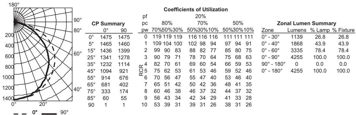
**2AVL4 50L MDR LP835**, 5095 delivered lumens, test no. 69071P9, tested in accordance to IESNA-LM79.
