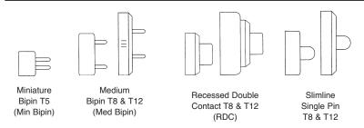
Bulb Shapes (Not Actual Sizes - Letters indicate the bulb shape while numbers indicate the diameter of the bulb in eighths of an inch.)
