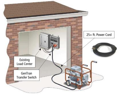
**IMPORTANT** This product must be installed by a professional electrician familiar with residential or commercial electrical wiring and building codes. This system must be installed in accordance with all national and local codes and ordinances. Never operate a generator indoors or in an enclosed area. Make sure generator is at least 5 feet away from any door or window opening!
