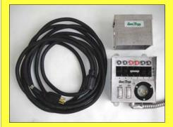
The 2002 National Electrical Code mandates that a transfer switch be installed with ALL standby power systems, including portable generators. During a power outage, a transfer switch safely isolates those circuits using generator power from the rest of the house or building, so the danger of backfeeding the electrical utility is eliminated. All GenTran<sup>™</sup> transfer systems meet the requirements of Article 702.6 for Optional Standby Systems.
