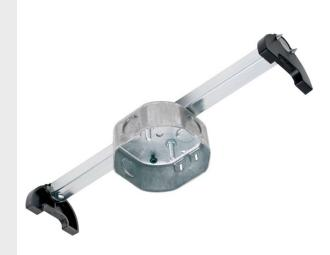
Fan Brace - Standard grade with standard box, single #10 support for 16-24" spans. 12 pack.
