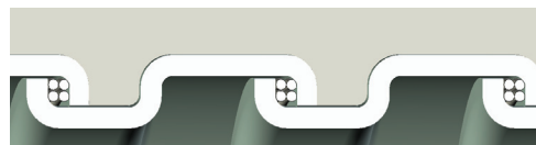
Square-Locked Design with cord packing 3/8" through 1-1/4"
