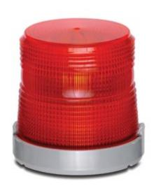
The 48XBRM Series LED Visual Indicator is a UL and cUL listed dual-mode signaling device housed in a corrosion resistant Type 4X enclosure. The 48XBRM Series XBR (XTRA-BRITE™) is suitable for indoor or outdoor installations, and can be panel or conduit mounted. The base is manufactured from a polycarbonate/ABS blend, and the lens is made of shatter resistant polycarbonate. The 48XBRM Series LED is available in AC and DC models with a gray base, and an amber, blue, green, red or white lens.
