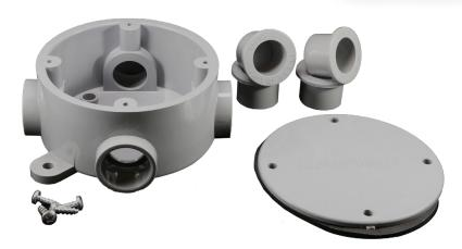
Round Junction Boxes are designed to support electrical devices and fixtures. They also provide necessary protection for wires and terminals. They are 4" round enclosure with four entrance hubs. Round Junction Boxes are surface mounted to walls or ceilings to terminate conduit runs or join two to four conduits at a common point.
