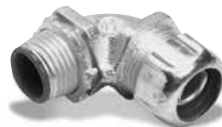
Malleable iron, tapered hub threads. With safe-edge ground cone and double bevel sealing ring (through 2").
