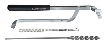
Klein's Flex Bit kit includes everything you need for drilling and pulling wire and cable in-wall. The flexible drill bit makes 9/16-Inch (14 mm) holes in wood. The folding placement tool helps guide the bit as you drill. The pulling grip attaches to the flexible drill bit after the hole has been made to pull wire and cable through.
