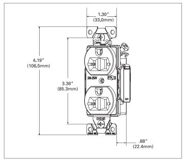
Figure 4. AH5462 Line art with dimensions
