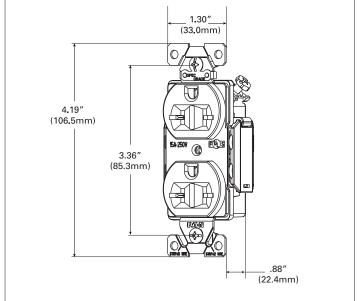
Figure 3. AH5662 Line art with dimensions
