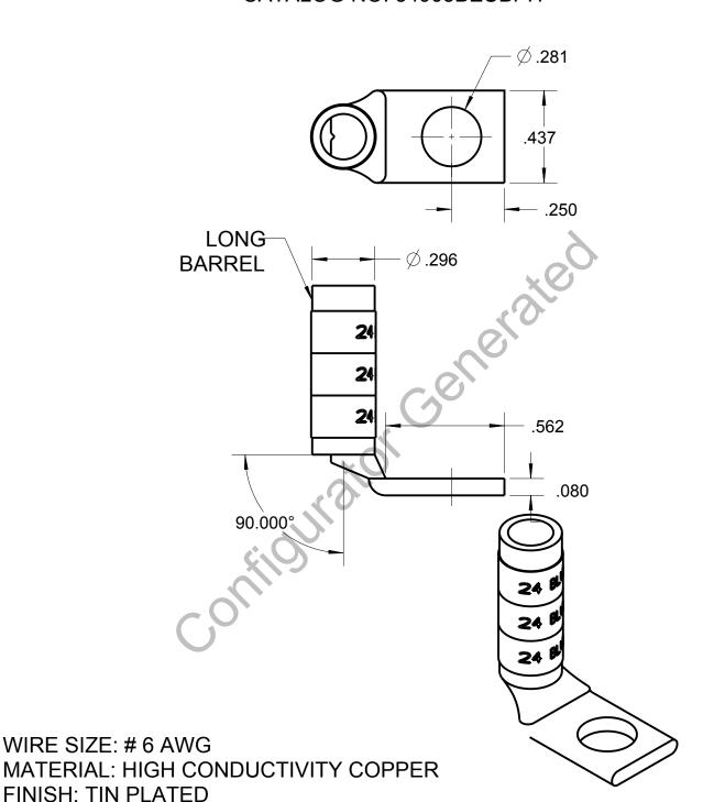
**GENERAL NOTES** ALL DIMENSIONS ARE FOR REFERENCE ONLY. 2. DIMENSIONS IN BRACKETS [] ARE IN METRIC UNITS. DESCRIPTION: 1 HOLE LUG REVISIONS SEE ERN ( \*\*\*\* ) DRAWING NO: WSD-003182 FOR APPROVAL SIGNATURES ORIGINAL PROJECT NO / (ERN NO) SHEET NO: REV. NO: & RELEASE DATE.
