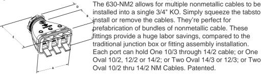
Download Photo Image Dimension A in Inches: 2.613 Dimension B in Inches: 1.350 Dimension C in Inches: 2.064 Dimension D in Inches: 0.471 Dimension E in Inches: 3.071
