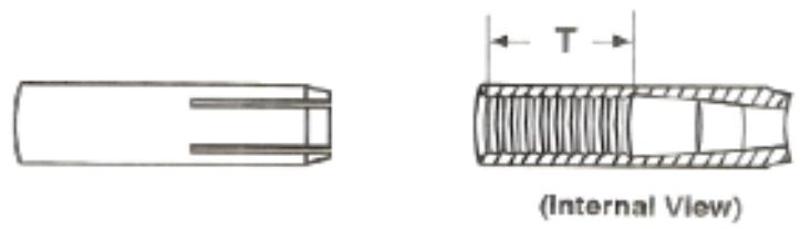
**Drop In Anchors are a two piece, internally threaded expansion anchor. The anchor is for flush mounting, medium to heavy duty applications in solid base materials such as stone or concrete.**
