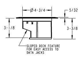
RECESSED FLOOR BOX INCLUDES ACCOMODATION FOR ONE RECEPTACLE (DUPLEX OR GFCI) AND TWO STANDARD KEYSTONE STYLE DATA JACKS (RECEPTACLES AND DATA JACKS ARE NOT INCLUDED).
