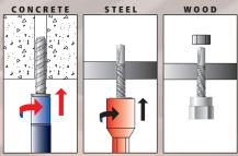
Thread the appropriate diameter steel threaded rod or threaded bolt into the coupling. The threaded rod or bolt should fully engage the thread length of the coupling on a vertical mount fastener. The threaded rod or threaded portion of the bolt can pass through coupling of a side mount fastener.
