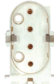
80-1602 Shunted Vertical Snap-In Mounting for Electronic Ballasts, Side Push-In Wiring Wireways Allow Routing on Top or Bottom of Mounting Panel 2" H x 1 1/4" W x 7/8" Dia. 660W-600V
