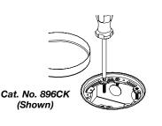
Step 2 Place the gasket over the floor plate and attach the cover using (3) #8 flat head screws.
