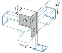
Page Notes:  $\frac{1}{4}$ " thick,  $\frac{15}{8}$ " wide, holes  $\frac{9}{16}$ " dia., spaced  $\frac{17}{8}$ " on center and  $\frac{13}{16}$ " from end.
