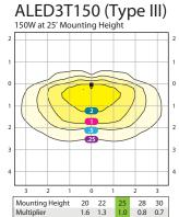
**Type III:** Ideal for roadway, general parking, and other applications where a larger pool of light is required. Usually located near the side of the area, allowing light to project outward and fill area.
