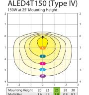
**Type IV:** "Forward Throw" is especially suited for mounting on the sides of buildings and walls, and for illuminating the perimeter of parking areas. It produces a semicircular distribution.
