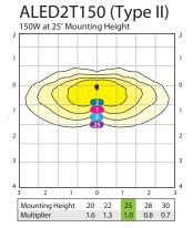
**Type II:** Ideal for wide walkways, on ramps, bike/jogging paths and other long and narrow applications. Meant for lighting larger areas and usually located near the roadside.
