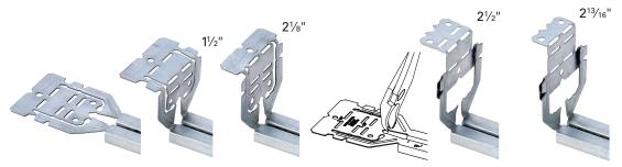
• Box mounting clip attaches to electrical box to bracket without hardware
